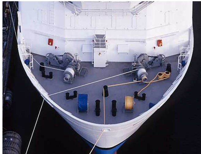
Anchoring, mooring and towing systems A typical arrangement on the fore deck of a passenger vessel
