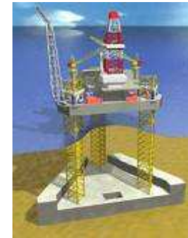
TPG 500 MFC Multi Field Concept with integrated oil storage
