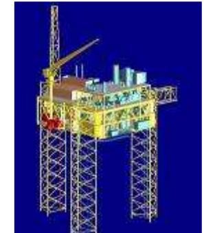
TPG 500 Trussdeck – Barge installed integrated deck with TPG 500 legs
